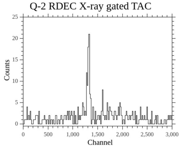
Fig. 2 Double charge exchange (Q-2) time spectrum from x rays in the RDEC energy region for 2.21 MeV/u  $F^{9+} + N_2$  (8 mTorr).
