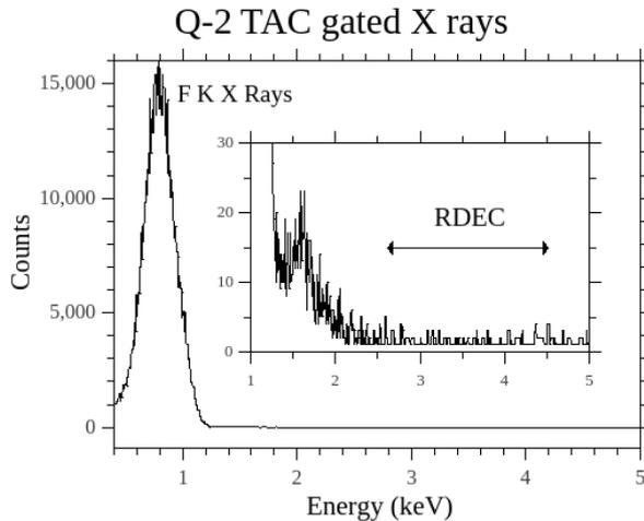
Fig. 1 X-ray spectrum associated with double charge exchange (Q-2) for 2.21 MeV/u  $F^{9+} + N_2$  (8 mTorr).
